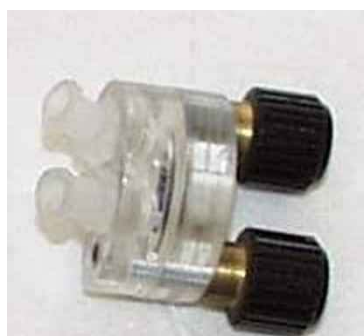
Figure 4. Plexiglas chamber utilized during the flow analysis of protein-protein interaction: the upper part, with the flow inlet and outlet, allowed the easy insertion of the biological fluid to be analysed and the lower allowed the proper housing of the quartz.
