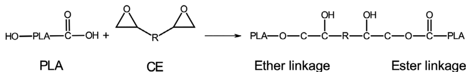
FIG. 4. Generalized reaction mechanism of a multifunctional epoxy chain extender with the hydroxyl and carboxyl end groups in PLA.
